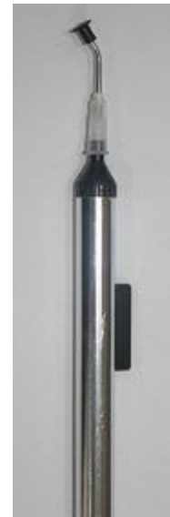
Fig.2_porcelain laminate suction holder
